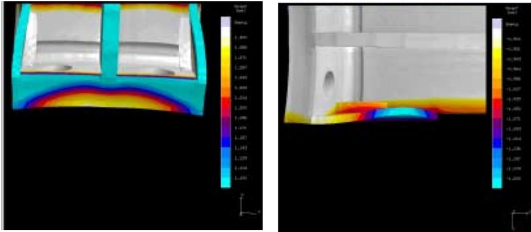
Figure 16 – Simulation and measurements (below) of anisotropic shrinkage and warpage
